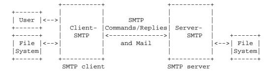
When an SMTP client has a message to transmit, it establishes a two-way transmission channel to an SMTP server. The responsibility of an SMTP client is to transfer mail messages to one or more SMTP servers, or report its failure to do so.
